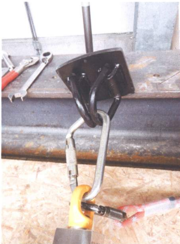
Fig. 11, test layout 1: attachment eyelet at steel construction
