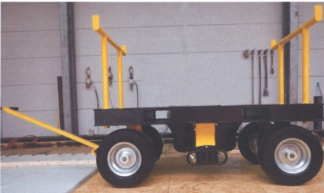
Fig. 8: anchor device type attachment eyelet, mounted at fall safety cart and placed on a surface resembling the structure (here: OSB surface)
