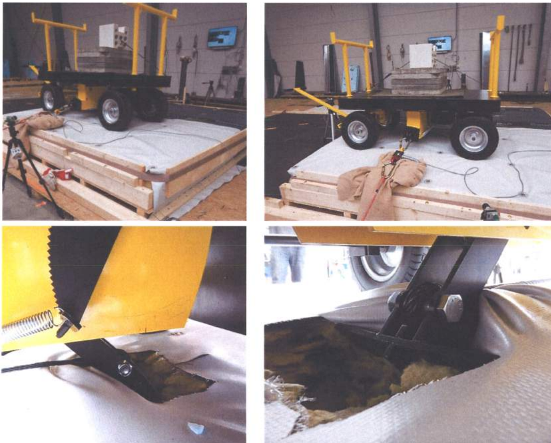
Fig.: 27-30, test layout 6: safety cart on PVC foil and rockwool
