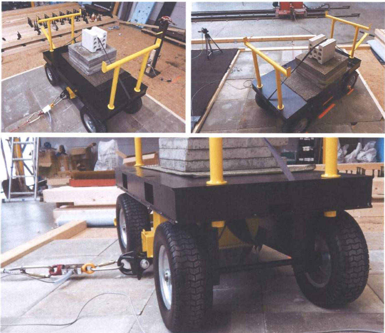
Fig. 20-22, test layout 4: safety cart on concrete
